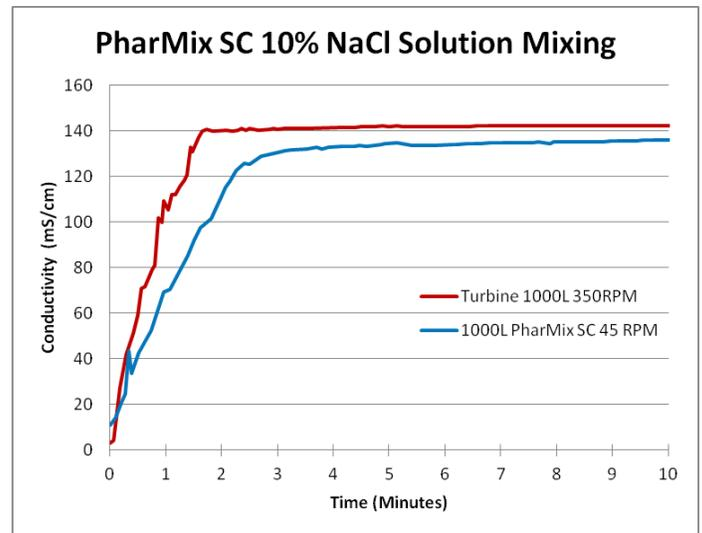
Based on the conductivity testing, one can see that the PharMix SC System is fully capable of consistently dissolving a 10% salt solution in less than 5 minutes in either a 200L or scaled up 1000L volume. It also shows that the conductivity testing of a PharMix SC System or a conventional turbine prop mixer were nearly identical.
