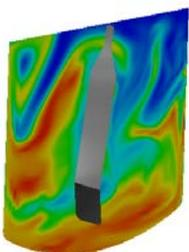
The first design phase was using CFD (Computational Fluid Dynamics) to try to get the feel for the mixing capability of the PharMix SC System. This was compared to conventional axial turbine props that were also analyzed using CFD. The system was built and tested using beads of different specific gravities to optimize the mixing motion using the mixing paddle. The final tests were pH indicator and 10% salt solution testing. The following chart shows the systems that were compared.
